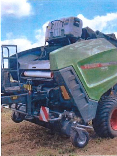
FIGURE 4 PRESSE AVEC INJECTEURS D'ACIDE
